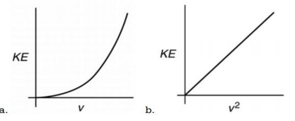
Kinetic Energy (KE)= 1/2mv<sup>2</sup>, so it makes sense that since KE is proportional to v<sup>2</sup>, that would give a straight line.
